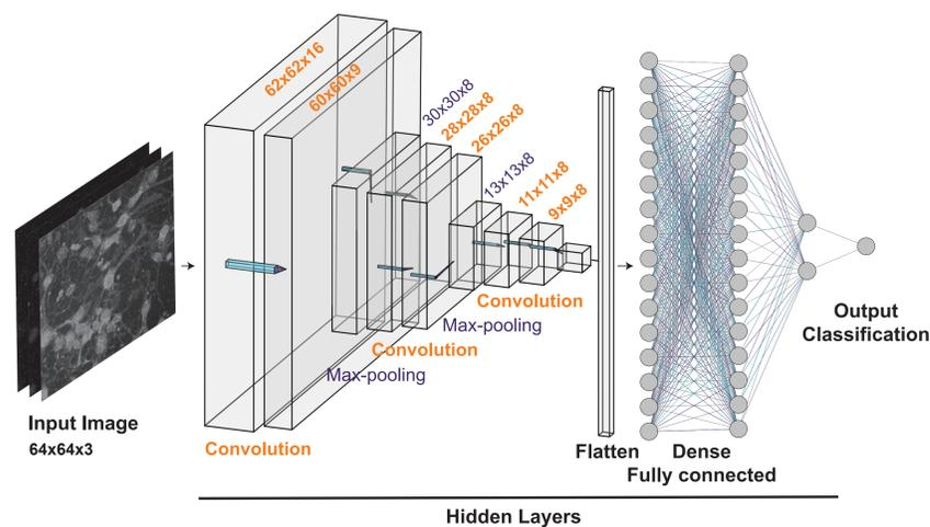
Schematic representation of the starting convolutional neural network. A simplified version of the VGG-16 model with 8 layers and 6042 trainable parameters. The dimensional outputs are indicated.
