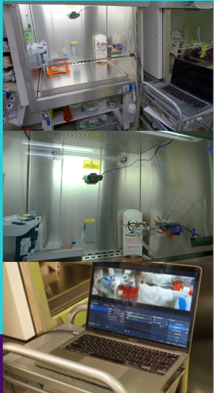
Image 1. Setup of Logitech webcams inside the hood and OBS software
